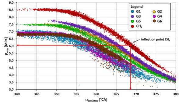
Fig. 6: The course of the maximal pressure depending on the angle at which 50 % of the fuel mass is burned. Conditions: 1500 rpm, full load, stoichiometric mixture.
