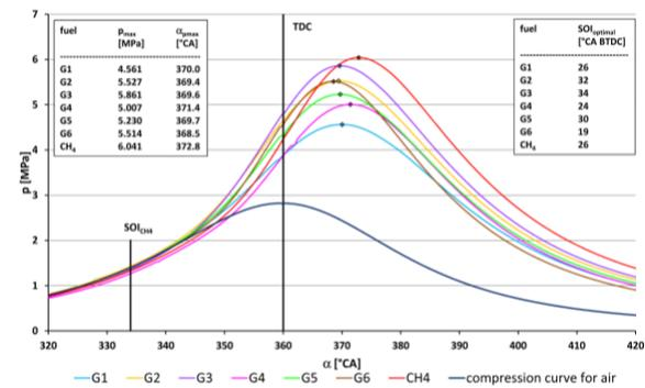
**Fig. 5: Pressure profile  $p$  in the cylinder of an internal combustion engine during operation on methane and synthesis gases (G1-G6). Conditions: 1500 rpm, full load, stoichiometric mixture, optimal start of ignition (SOI) angle for each fuel, compression curve is for air.**
