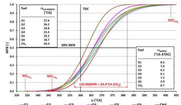
Fig.7: Course of fuel burnout as a dependent on the crankshaft angle for methane and synthesis gases (G1-G6)(MFB - Mass Fraction Burned,  $\alpha$  - Crankshaft Rotation Angle, TDC – Top Dead Centre, SOI – Start of Ignition, SOC – Start of Combustion, EOC – End of Combustion) Conditions:1500 rpm, full load, stoichiometric mixture, optimal SOI angle for each fuel
