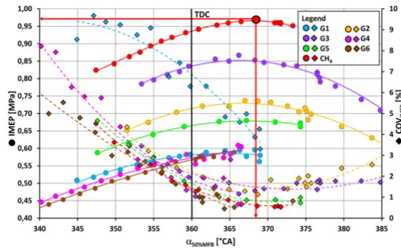
**Fig. 4: Course of the indicated mean effective pressure (IMEP) and coefficient of variation (COV<sub>IMEP</sub>) dependent on the angle of the crankshaft where the 50% of the fuel mass is burned ( $\alpha_{50\%MFB}$ ) for methane and researched gases (G1-G6). Conditions: 1500 rpm, full load, stoichiometric mixture.**
