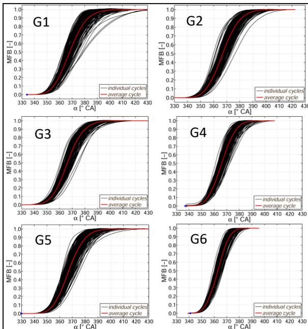
**Fig.8: The course of mass fraction burned (MFB) for measured synthesis gases (G1 – G6) at optimal start of ignition angle (conditions: speed 1500 rpm, full load, stoichiometric ratio, 197 consecutive cycles)**
